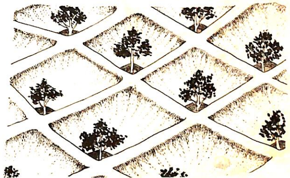
Figure 8-17: Micro-catchment with ground divisions
